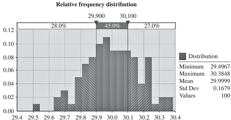
**FIGURE 19.18** Result of Monte Carlo simulation showing a relative frequency distribution of combined total length of three components A, B and C that individually have normal distributions of 5, 10 and 15 mm, respectively, each with a standard deviation of 0.1 mm. The mean expected combined total length is approximately 30 mm, but the simulation shows the variation around this, e.g., that only 45% of assembled components are expected to be within  $\pm 0.1$  mm of this mean value.
