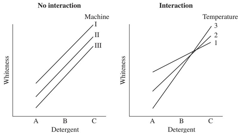
FIGURE 19.17 Interaction. (*Quality Planning and Analysis*, Copyright 2007. Used by permission.)
